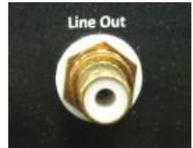
to connect to analog amplifiers. This output activates automatically any time the ZONEC2 receives audio streams. More detailed specifications include: *10k Ohm, unbalanced, 2Vpp line-level output.*
