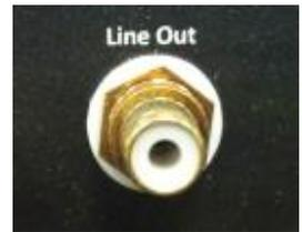
typically used to connect to analog amplifiers. This output activates automatically any time the ZONE-LO receives audio streams. More detailed specifications include: *10k Ohm, unbalanced, 2Vpp line-level output.*
