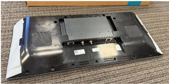
Remove included VESA mount and hardware package from box nested in protective foam endcap of packaging.
