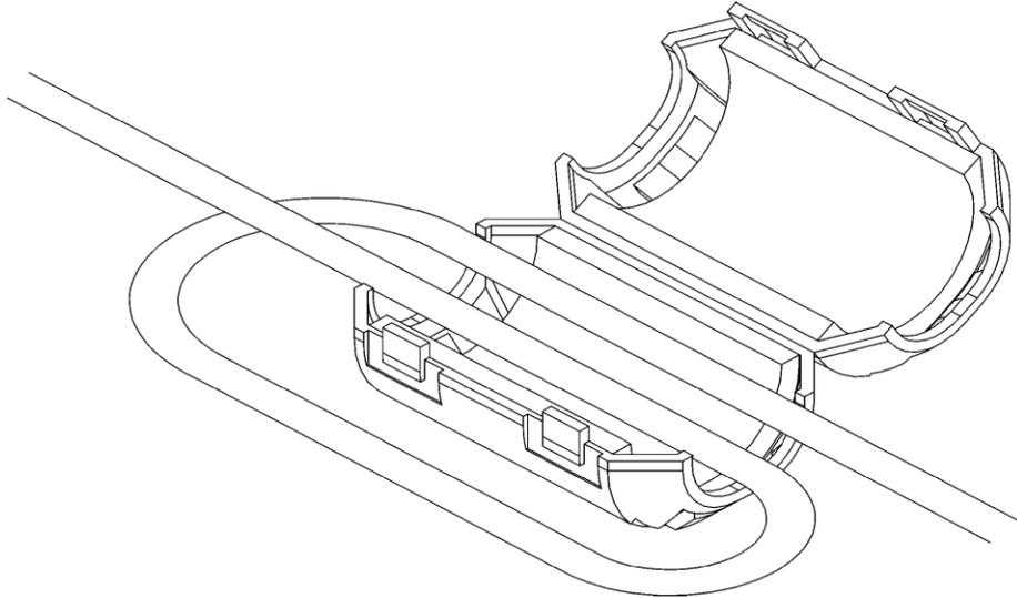
2. Take care not to pinch the cable or your fingers when closing and locking the ferrite core.
